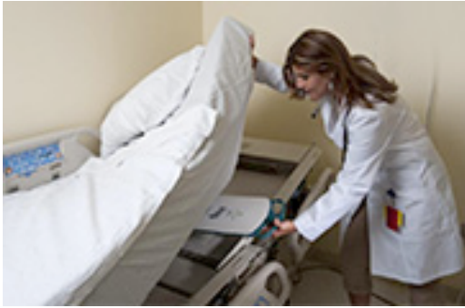
Fig. 6. Positioning of the Early sense sensing plate. SOURCE: [7].
