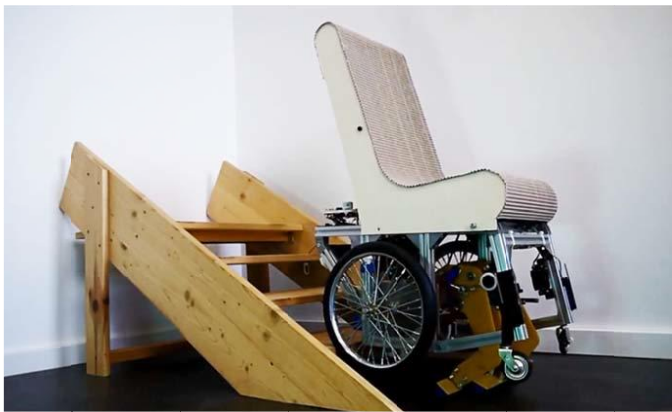
Fig. 2. The demonstrator model while climbing stairs; the legs are below the wheelchair and push it up.
