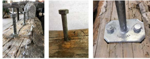
Fig. 7. Shear connectors after the test: (a) beam A, (b) beam B and (c) beam C.
