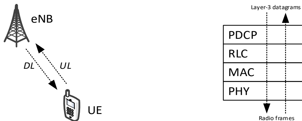
Figure 1. LTE-A radio access network (left); and protocol layering (right).
