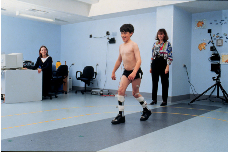
Figure 3.4 A child participating in a 3DGA in the gait laboratory. Two AMTI force plates are incorporated into the grey walkway. In the background there are two Vicon cameras mounted on the walls and a video camera on a tripod on the floor.
