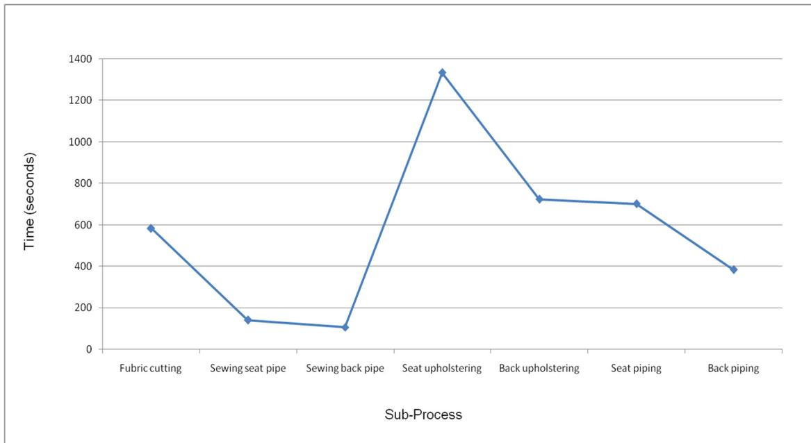
Figure 3.4 Time analysis of upholstery process for P1
