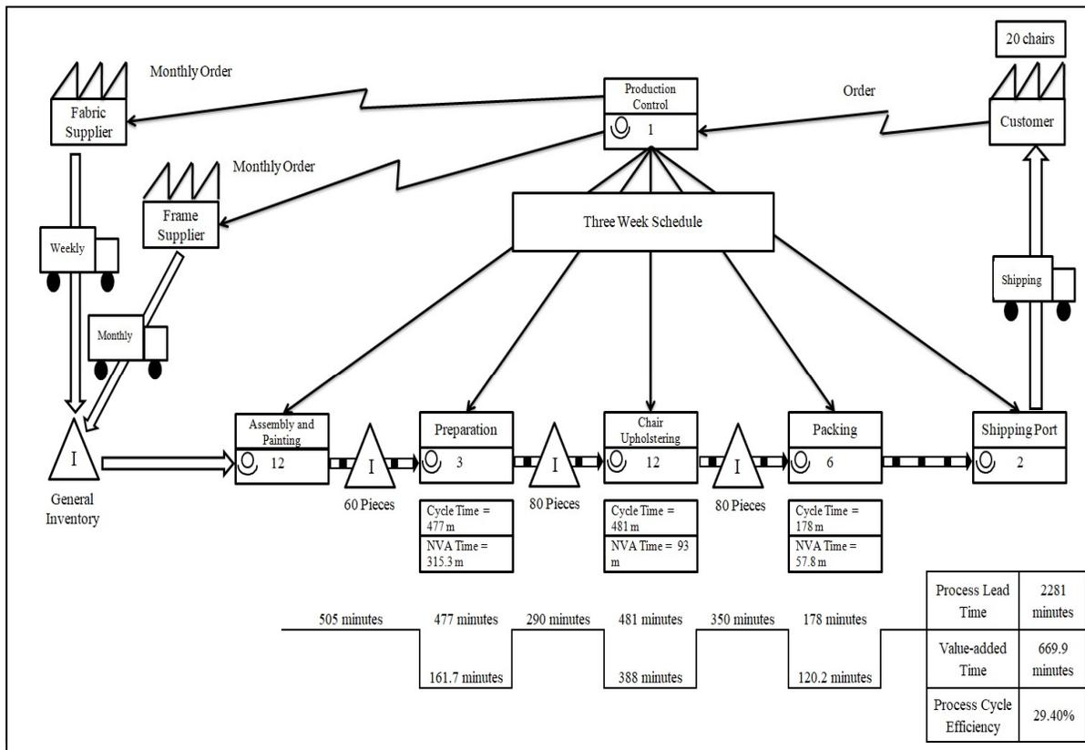
Figure 3.2 Current value stream map for P1
