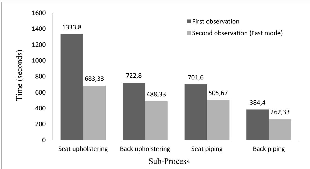
Figure 4.2 Comparison between two observations for upholstering operations
