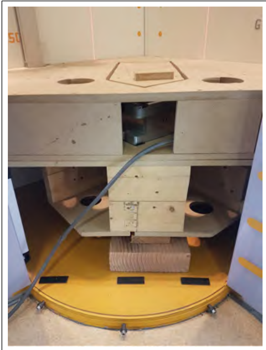
Figure 4-1: Force platform in the EOS® cabinet measures the forces under the studied foot in the middle while the contralateral foot is isolated from the force platform.
