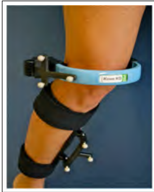
Figure 1-10 Anterior view of a right knee fitted with the KneeKG™ system. Secure fixation to the thigh and calf minimizes skin motion artifact.
