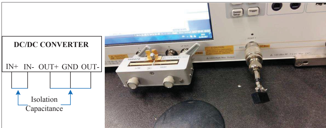
Figure 2.11 DC/DC converter isolation capacitance measurement
