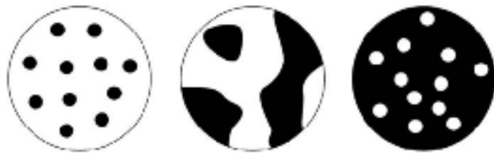
FIG. 1.1 Evolution of a blend morphology as a function of concentration [1]
