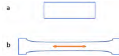
FIG. 6.1 Scheme of the specimens (a) before and (b) after elongation. The double arrow represents the cut for SEM observations.
