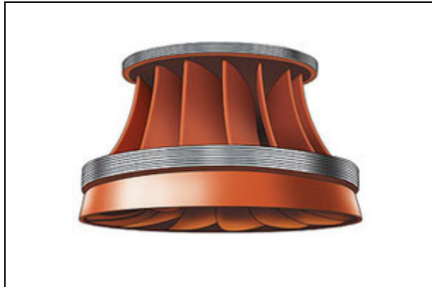
Figure 1-1: Turbine Francis (tiré de http://www.hydroquebec.com/comprendre/hydroelectricite/types-turbines.html )
