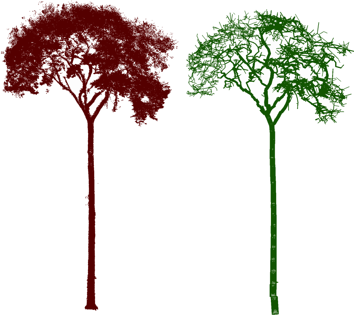
Figure 2.2: Example of one tree TLS point cloud from Guyana dataset (left, in dark red), and the same tree modelled by QSM (right, in green). Figure from (Gonzalez de Tanago et al., 2016).
