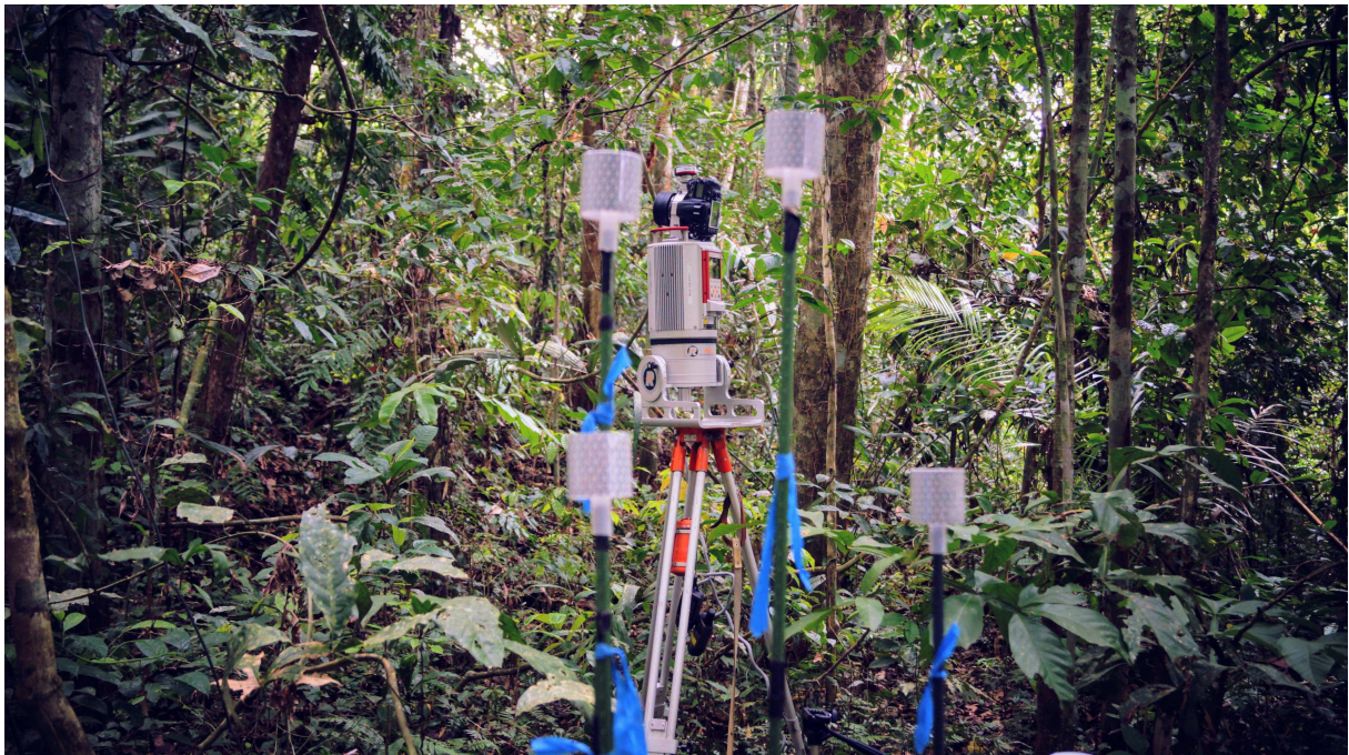
Figure 1.2: RIEGL VZ-400 terrestrial LiDAR mounted on a tripod surrounded by 5 cm cylindrical reflectors in Madre de Dios, Peru.
