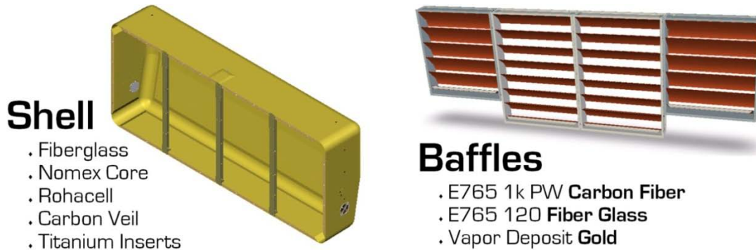
Figure 12: Composite Materials are used to fabricate the IEC
