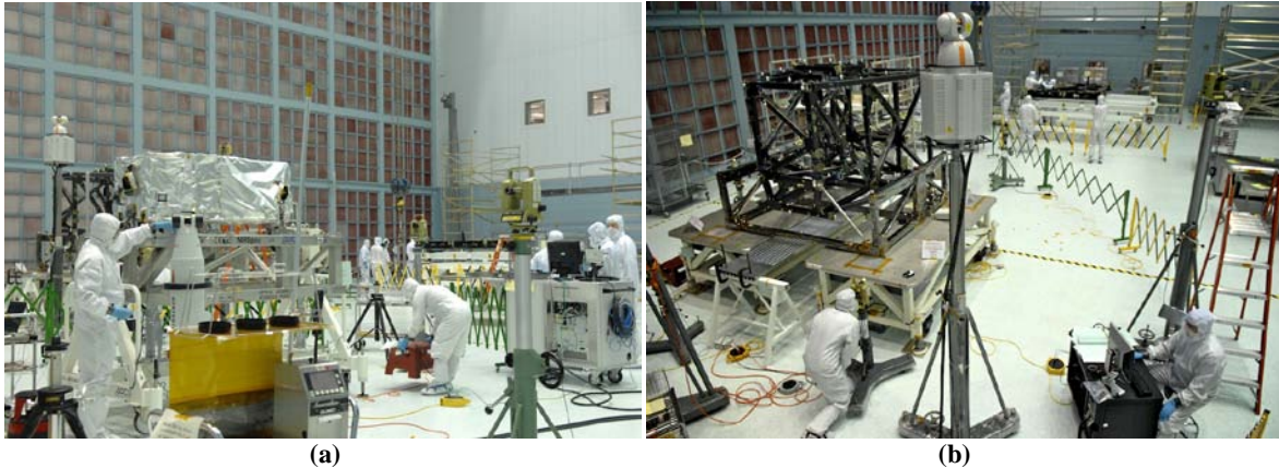
Figure 24: a. The ETU NIRSpec instrument (middle, left) during post-shipment metrology operations. b. Foreground: The ISIM Structure (left) undergoing coordinate system metrology using LIDAR and theodolite instruments. Background: The ITP is being readied for cryogenic testing.
