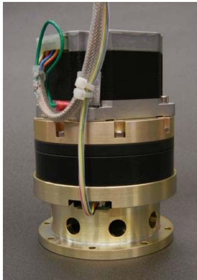
Figure 8 Photograph of the tilt-axis gearmotor assembly
