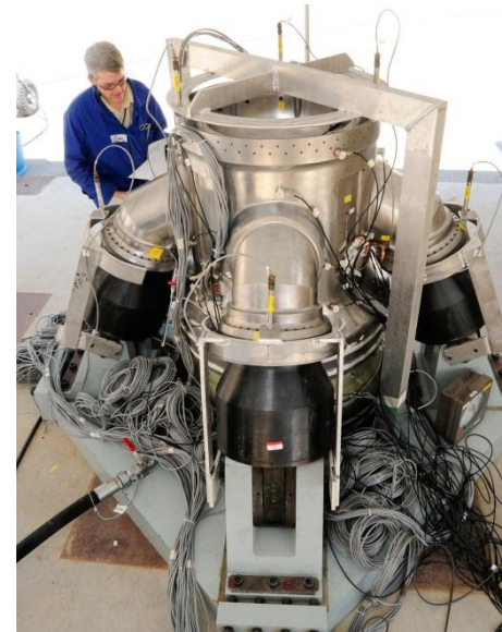
LAS AM manifold during hydroproof testing at ATK
