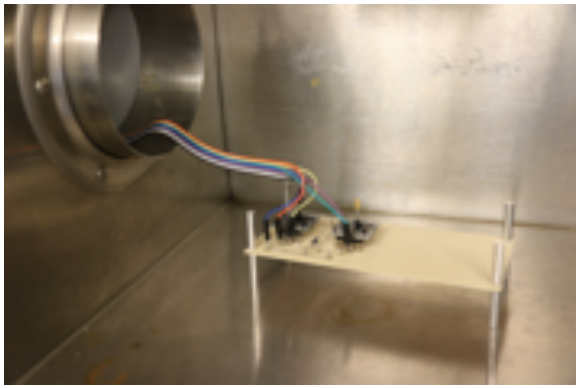
Figure 2. Two PNI Sensor Corporation induction magnetometers in a thermal chamber undergoing testing.
