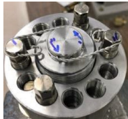
Figure 12.—Supernut-separation bolt safety multiple-wire configuration using proper horizontal alignment with correct winding direction around a large-diameter center post.
