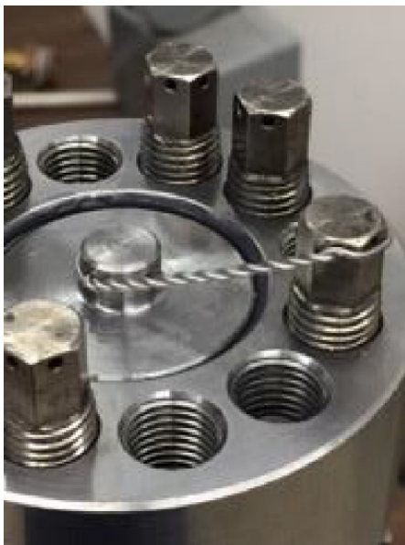
Figure 9.—Supernut-separation bolt safety wire configuration used during structural test article vibration test. Note the relatively small diameter center post and incorrect (backward) winding direction around the center post.
