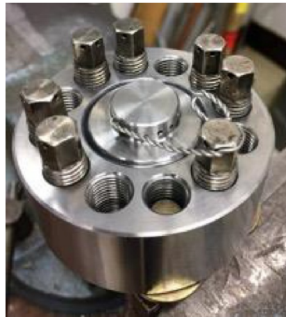
Figure 11.—Supernut-separation bolt safety wire configuration using improper angled alignment with correct winding direction around a large diameter center post.
