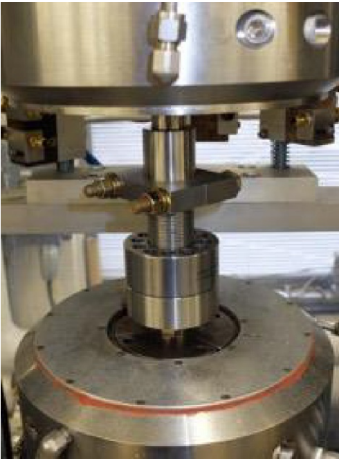
Figure 8.—Supernut-separation bolt loaded in load frame to measure prevailing (thread friction) torque.
