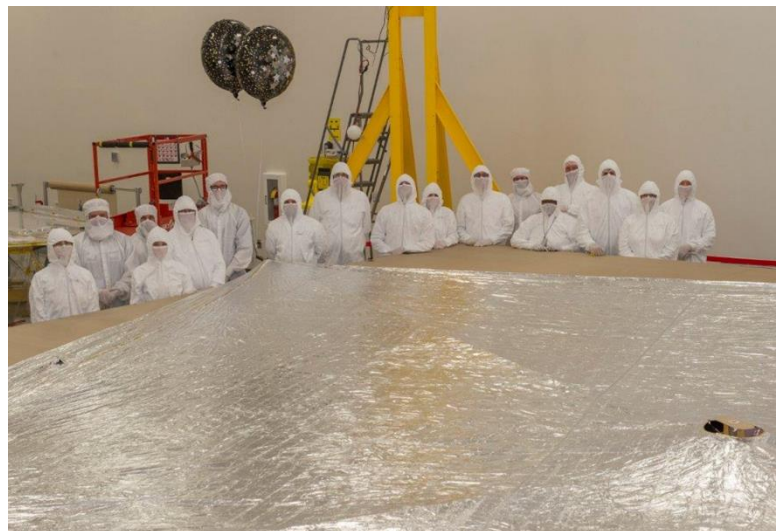
Figure 3. The NEA Scout's 86 m 2 solar sail was successfully deployed in a recent test near NASA's George C. Marshall Space Flight Center.
