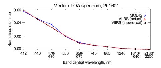
**Figure 4.** Median spectral observed TOA Sun-normalised radiance for MODIS (blue) and VIIRS (red) bands, and (black dashed) modelled expected VIIRS signal, after the AOD estimation and filtering steps described in Section 3.3.3. Data are from January 2016.
