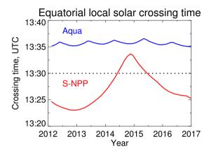
**Figure 8.** Variation of S-NPP (red) and Aqua (blue) satellite Equatorial local solar crossing times for the ascending (daytime) orbital nodes. The dashed line indicates the nominal 13:30 UTC crossing time often used as shorthand when discussing these platforms.
