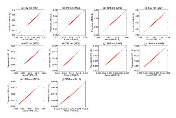
Figure 5. Bin-median observed and theoretical predicted VIIRS TOA Sun-normalised radiance  $(L/E_0)$  for suitable matched pixels in January 2016. The dashed line indicates a 1:1 relationship.
