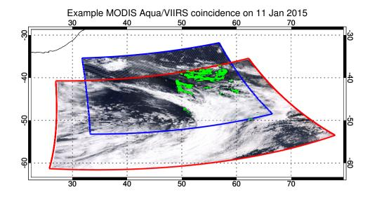
**Figure 2.** Example MODIS/VIIRS match up for two near-coincident granules (beginning one minute apart). The S-NPP VIIRS granule is outlined in red, and MODIS Aqua in blue. Suitable matched pixels are shown in green.
