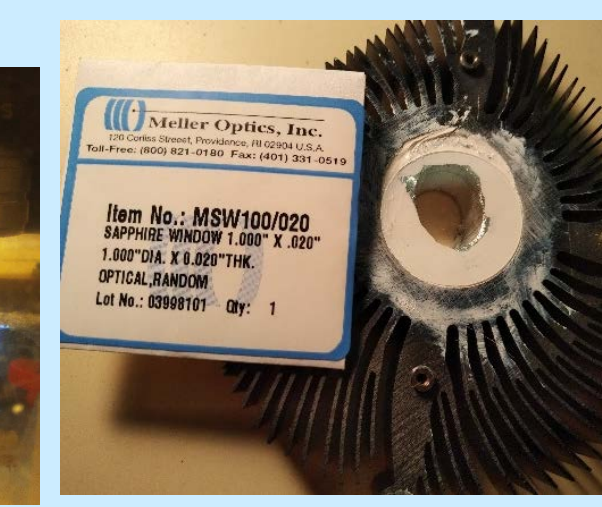
Sapphire window design (left); Milling COTS heatsink (center); Final product (right)
