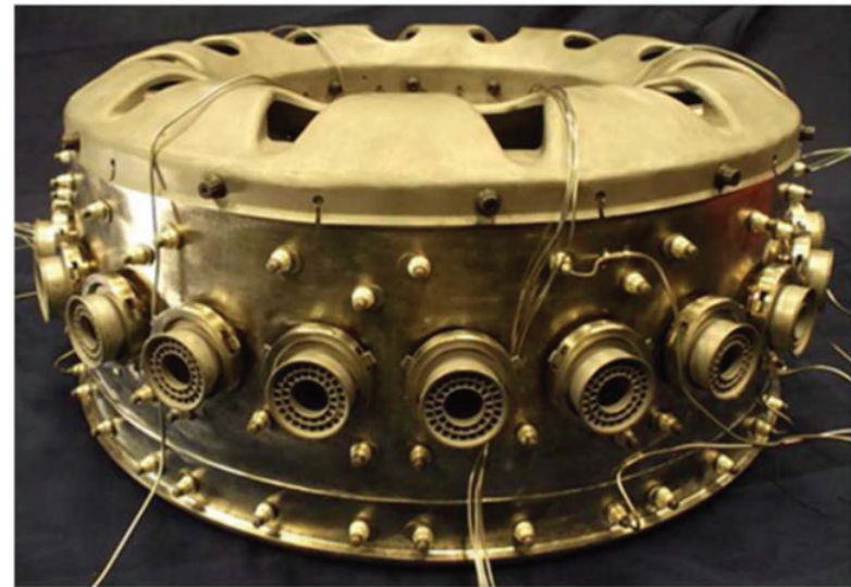
P&W ACS Annular Combustor
