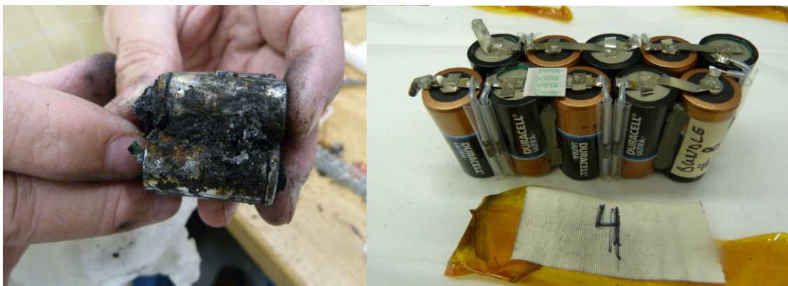
Figure 7.4-9. Test #1 Post-test Images of Exemplar Cells from 4S Bundle Side (left) and from 10S Bundle Side (right)
