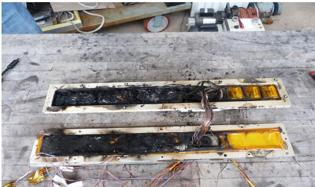
Figure 7.4-27. Test #4 Post-test Image of Open Battery Pack
