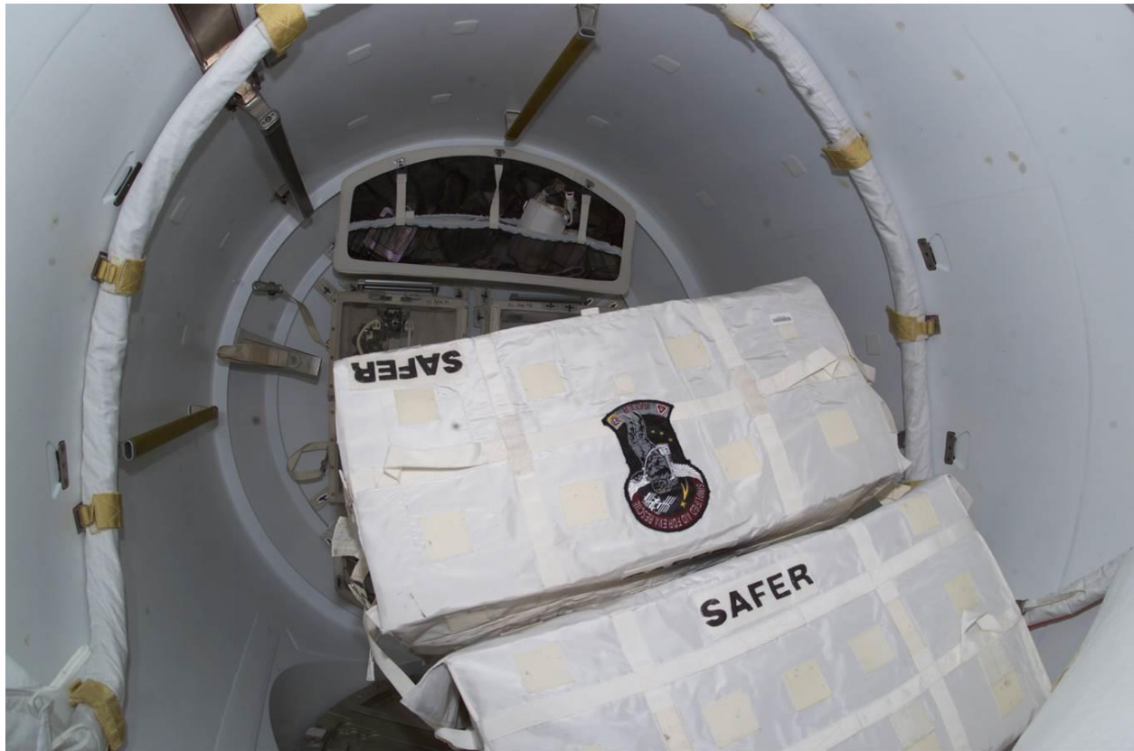
Figure 6.1-3. On-orbit SAFER Battery Assemblies in their Stowage Bags
