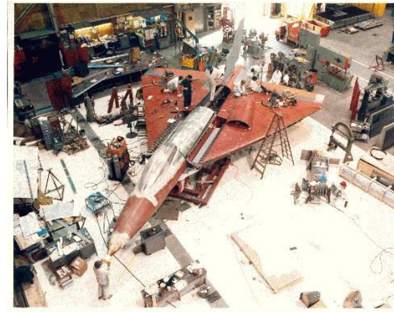
The E-7 Ejector Concept Under Construction
