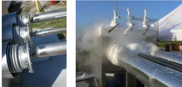
Figure 5. The thermal end guards and test pipe terminations of the cold pipe tester are shown without insulation (left) and with insulation during a test (right).
