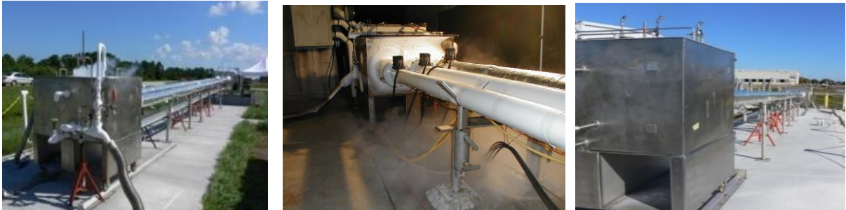
Figure 6. Overall views of the cold pipe tester Cryostat-P100 in operation.
