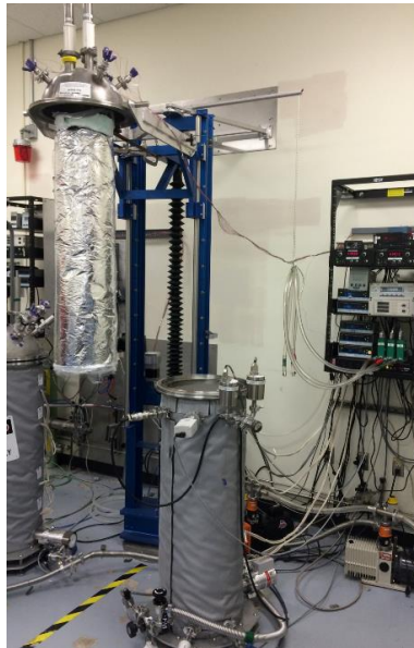
Figure 3. Cryostat-100 during test specimen installation (left) and cooldown operation (right).
