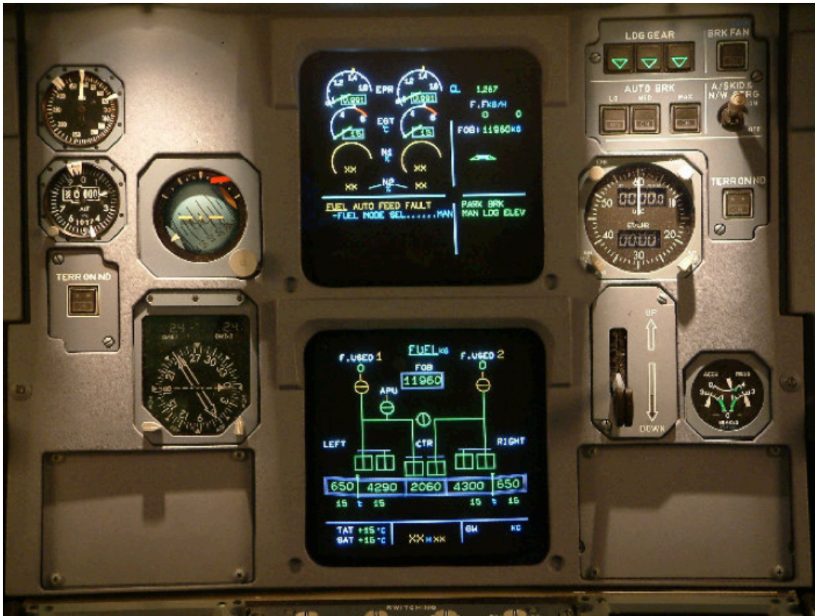
Figure 5. Airbus ECAM displays.
