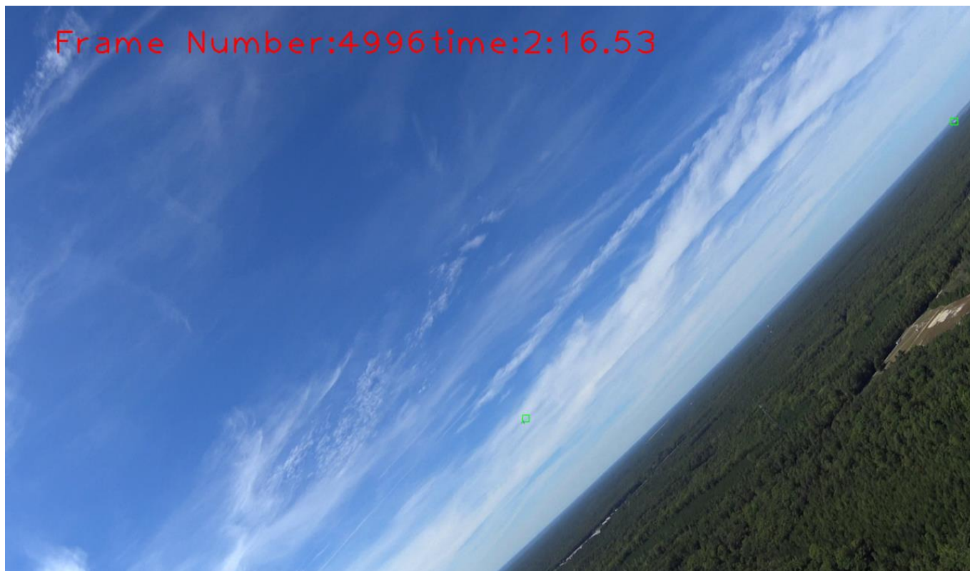
Figure 11: Detection limited to above horizon. To mitigate for false positives from the frame shown in 1, an image mask is used to limit detection to above the horizon. The result is a more robust “above the horizon sUAS detector”.
