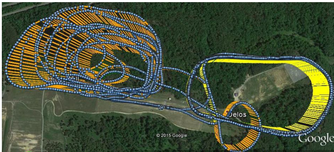
Figure 4: Flight Paths for MigCC vs SR22. The MigCC is on the right with the yellow elevation lines and the SR22 is on the left with the orange vertical lines. Note that the SR22 is in pilot in command mode and the MigCC is in AutoNav mode. The SR22 violates the buffer zone only on takeoff and the MigCC takes off only after the SR22 has reached its established altitude.
