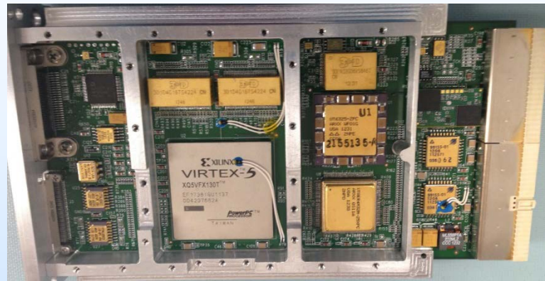
SpaceCube V2.0 Processor Card
