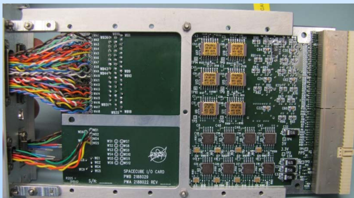
Restore-L Video/Spacecraft Interface Card
