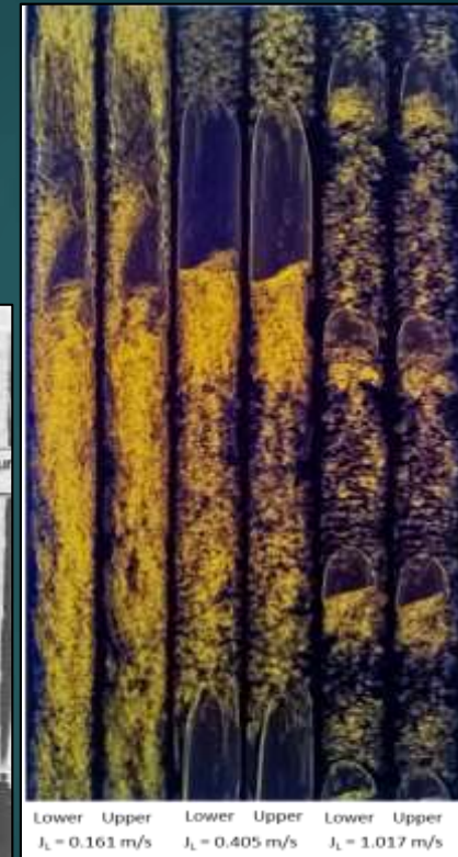
Virtual three dimensional plots of two phase flow obtained using X-ray CT. (Source: Reference 12)
