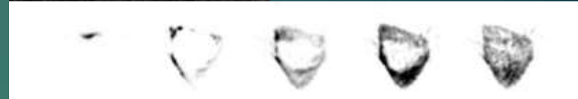
Visualization of pharmaceuticals progressively mixing in 0.3 m diameter steel drums (above) – 20 minute acquisition. (Source: Ref. 5)
