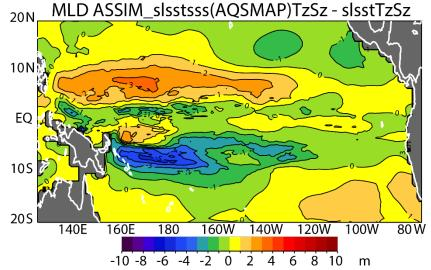
D<sub>20</sub> (for thermocline depth) Deepening the D<sub>20</sub> just off the equator Shoaling near the equator
