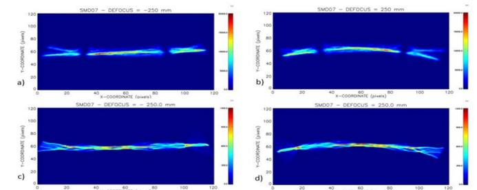
Panels a) and b) depicts intra-focal images measured ±250 mm from the focus of the telescope. Panels c) and d) show simulated intra- and extra-focal images generated at ±250 mm from the focus of the telescope. Obscurations of the spacers are not included in the simulated images
