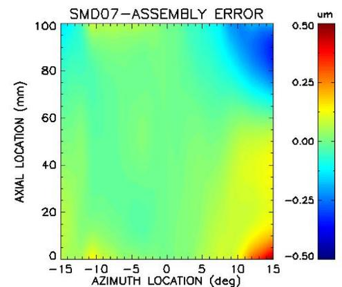
Assembly errors needed to match ray traced centroid and HPD variation of the model to measured centroid and HPD variation data
