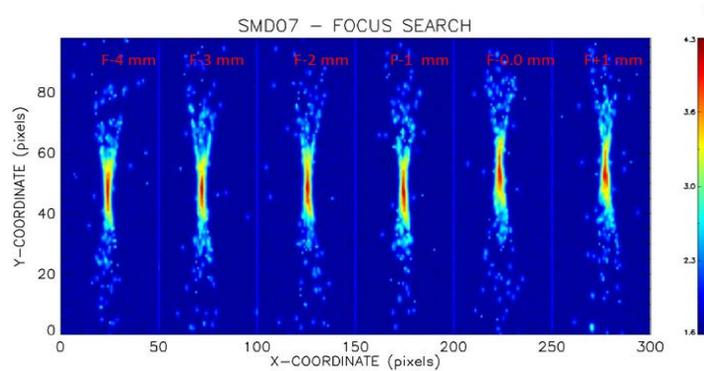
Focus search data at 4.5 keV measured in GSFC 600-m long beamline
