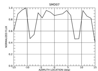
Flux variation measured across the azimuth of the mirrors. Mirror spacers block the x-rays at ~7 degrees from the edges and the edge points cover only half of the surface area
