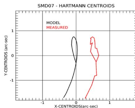
Plot shows measured centroids calculated from PANTER x-ray data and model centroids calculated from low order surface models. Model includes cone-angle, yaw, pitch, and de-focus errors.
