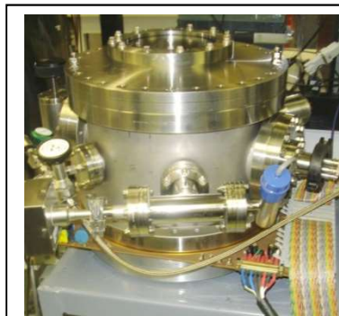
Figure 8 – Test chamber for out 10 cm MWD testing. A viewport is on the top of this chamber and source manipulation arm on the right. A printed circuit board provides support for the 3-DTI module under test.
