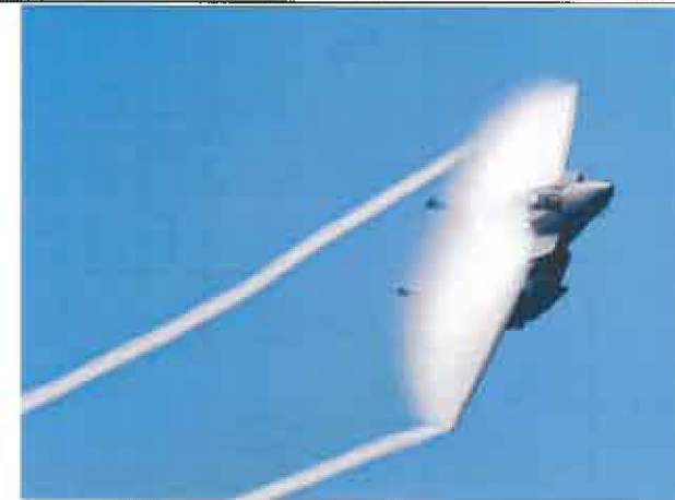
Elliptical Spanload and Wingtip Vortices
