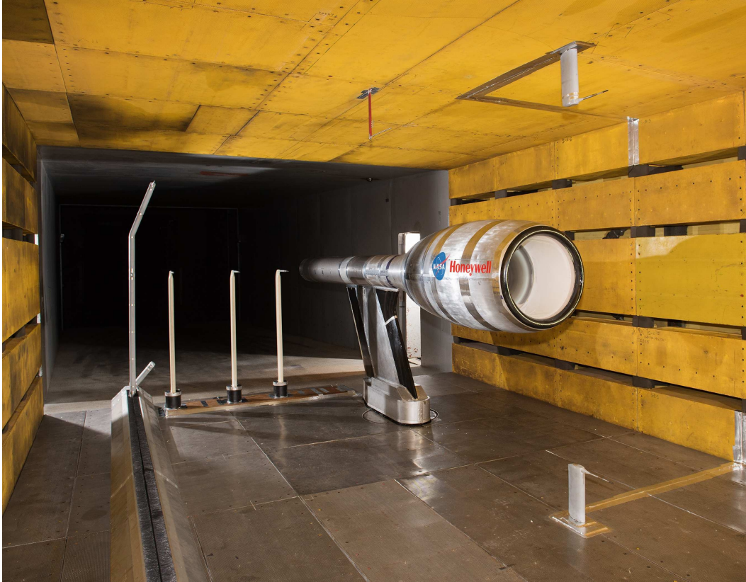
Figure 2: Example of a typical fan test in 9x15. A gray traversing probe holder with three microphones is shown on the far left of the image. Three fixed microphones are mounted to white probe holders between the traverse track and the fan rig strut. Upstream microphones mounted to floor and ceiling in front of fan. NASA GRC Image C-2014-8260.
