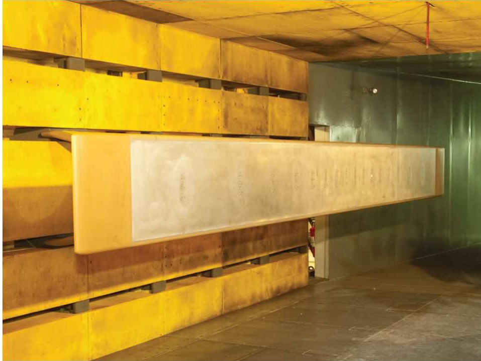
Figure 11: Linear array of flush-mounted microphones.
