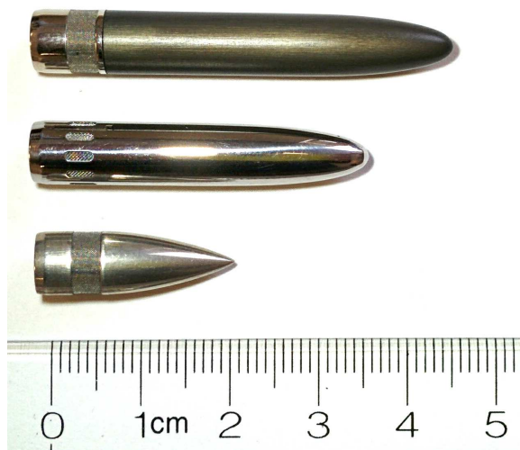
Figure 6: Three aerodynamic microphone forebodies. Top to bottom: FITE, GRAS, Brüel and Kjær.
