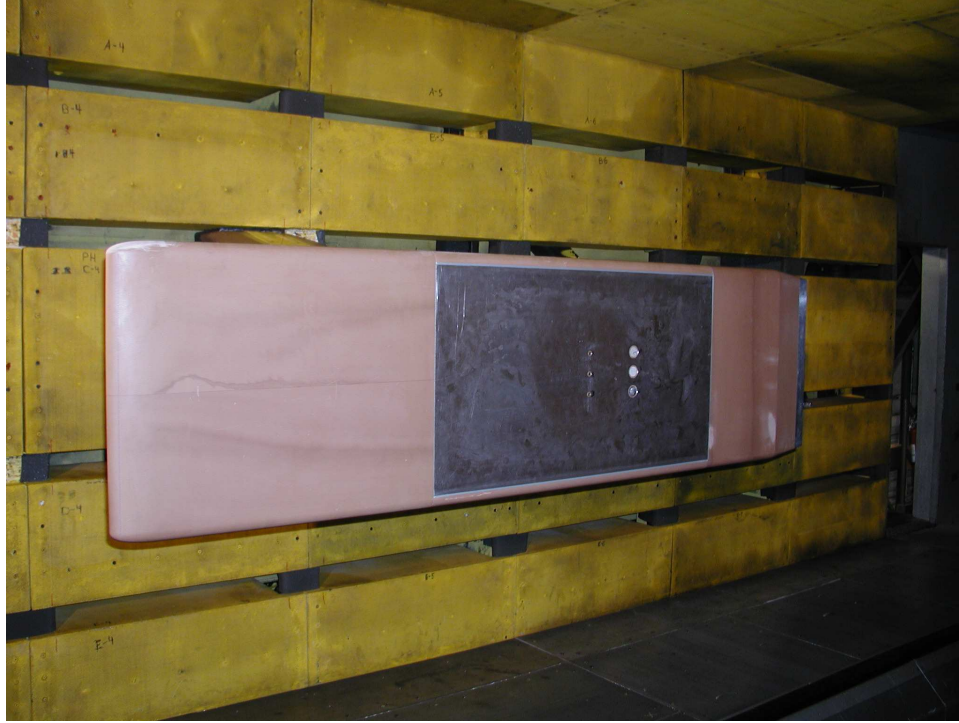
Figure 14: Linear array test article installed in the 9x15 LSWT.
