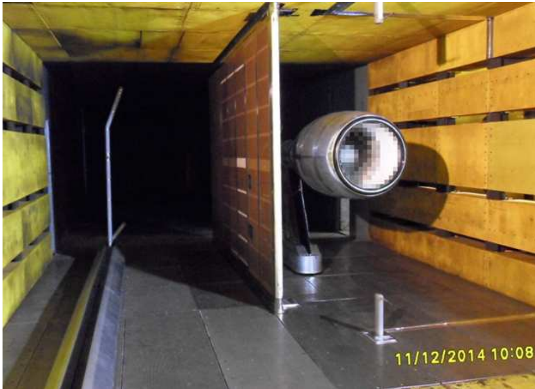
Figure 18: Barrier wall installed in the 9x15 LSWT.
