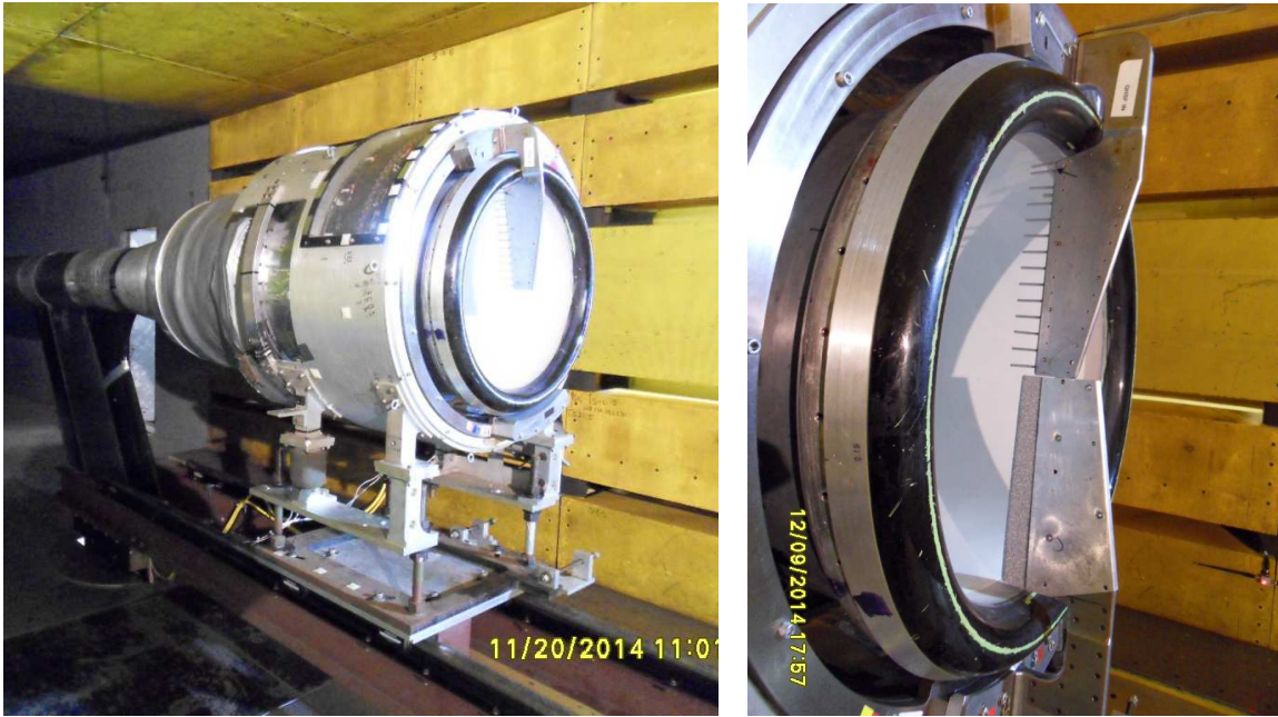
(a) Rotating rake installed over a fan model in the 9x15 LSWT. (b) Close view of dual rotating microphone rakes.
