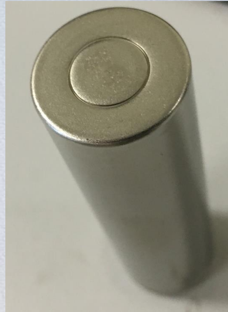
3.35Ah cell design, a bit more power capable than 3.5Ah design
