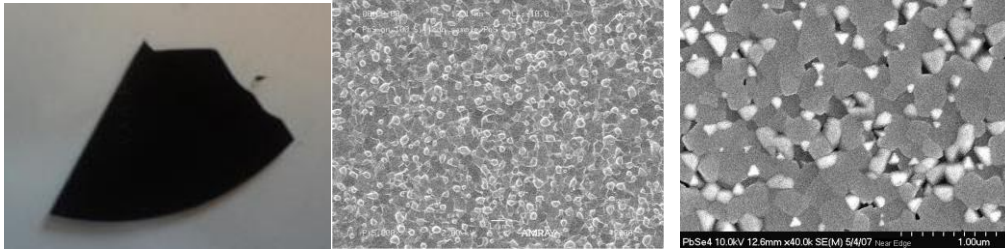
Figure 7. (a) film grown on Silicon substrate (b) morphology at low DT showing uniform morphology and (c) large DT showing different shaped grains and nonuniformity.
