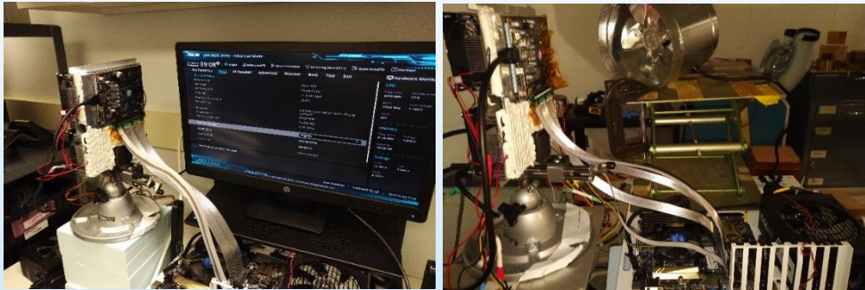
400W Cooling on Bare NVIDIA GTX 1050
