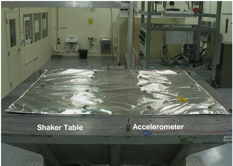
Figure 2. Shaker table experiment with aluminized MLI blanket.
