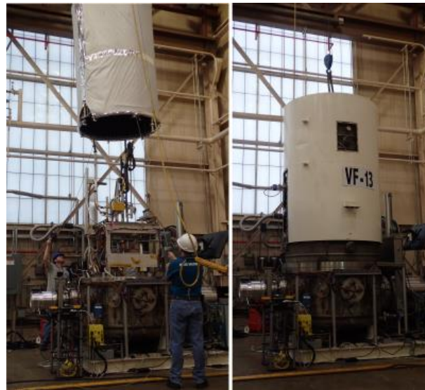
Figure 7. The VF-13 thermal vacuum facility at NASA GRC. At left, the RP hardware is visible as the cold wall is installed. At right, the 3.6 m tall chamber is sealed.
