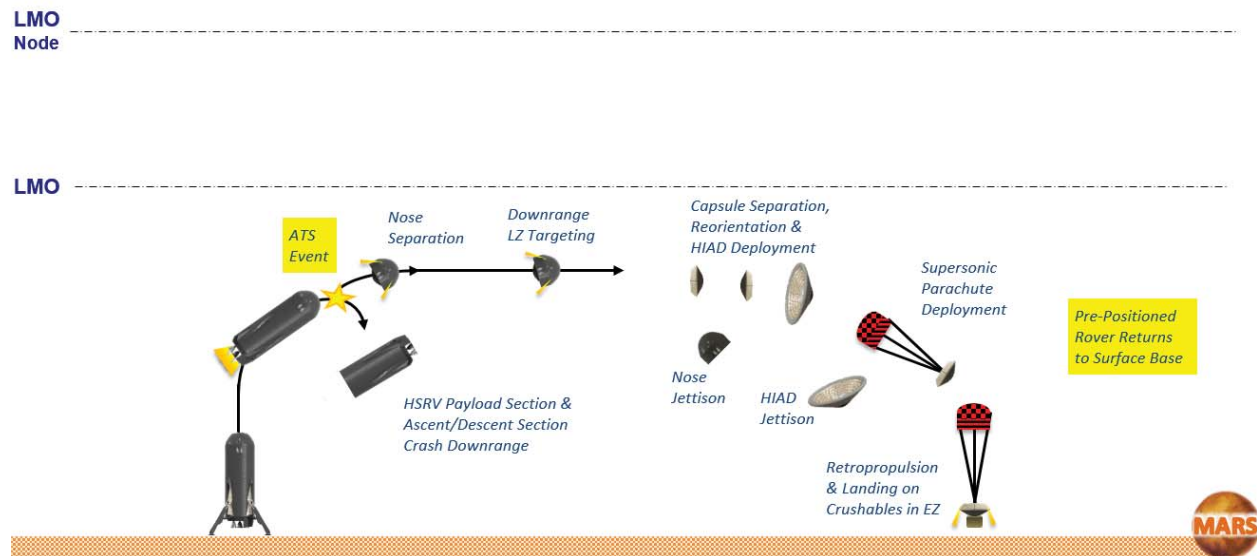
Figure 17. Concept of operation illustrating Mars ascent ATS targeting a common downrange location approximately 500 km east of the launch site using the capsule aeroentry and landing capabilities.
