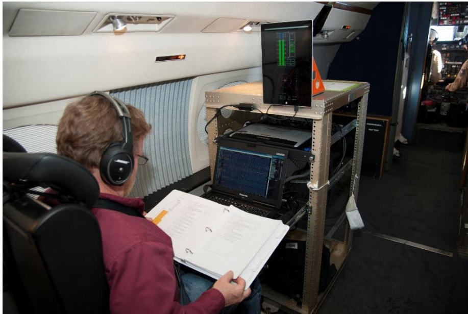
Fig. 15. Long-track and wake awareness display mounted in the cabin of the trail airplane.
