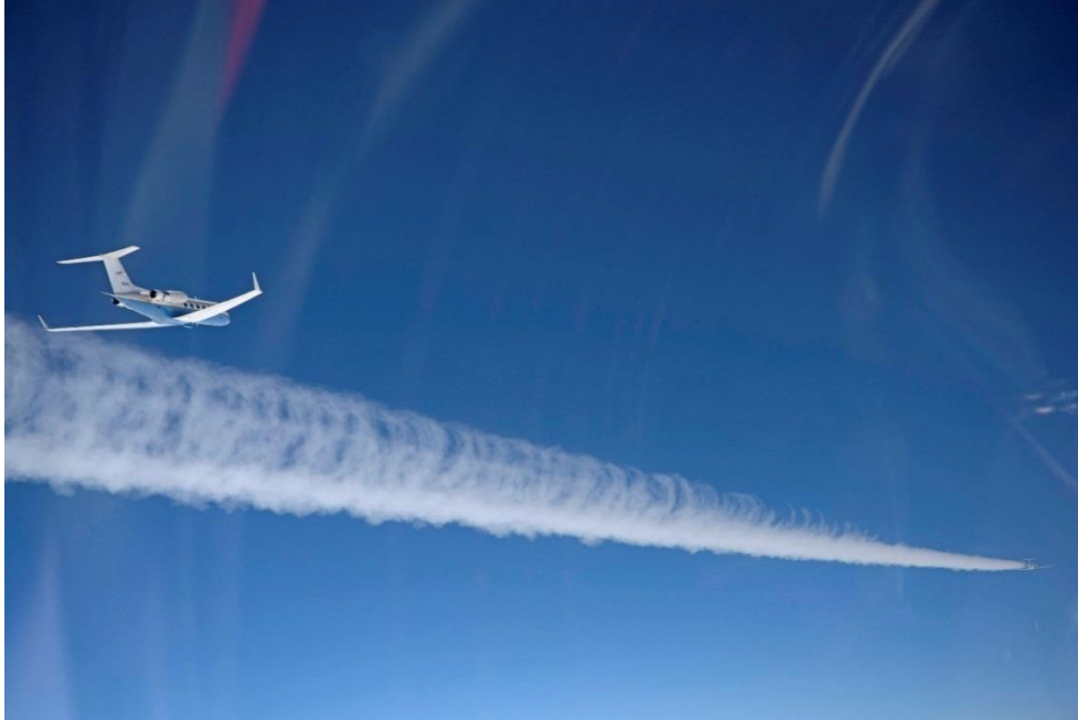
Fig. 12. Chase photo of the NASA C-20A airplane in formation with the wake contrails of the NASA G-III airplane.
