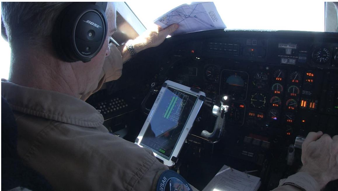
Fig. 13. Long-track and wake awareness display mounted on yokes, providing throttle cues to the pilot.
