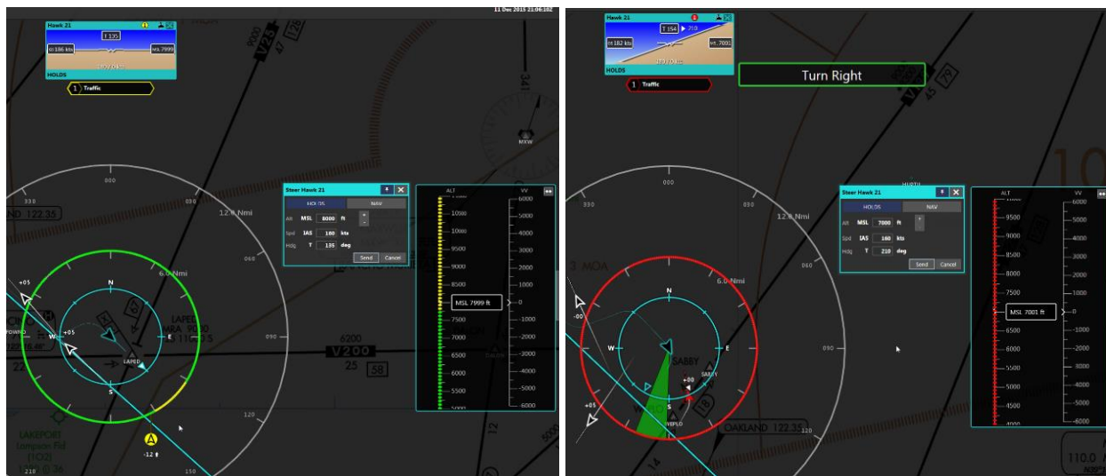
(a) (b) Fig. 1 Screenshots of the TSD with guidance to remain DAA well clear (a) and guidance to regain DAA well clear (b). As shown in (a), yellow bands on the inner range ring and altitude tape indicate headings and altitudes that are to be avoided. In (b), a green “wedge” and text box indicate the suggested maneuver.
