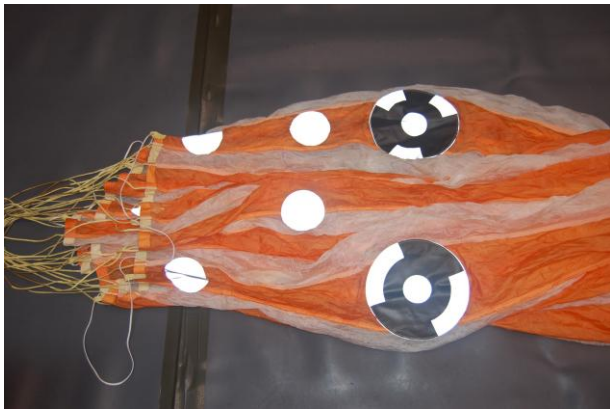
Fig. 4 Coded retro-reflective targets on LDSD canopy.
