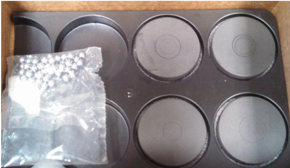
Figure 5. Test Specimens for low speed wear testing
