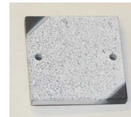
HfO 2 -Si, 50 h furnace cyclic, air
