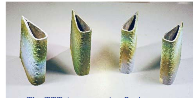
The TTT Augmentation Project Coated Turbine Vanes (Advanced EB-PVD NASA composition coatings)
