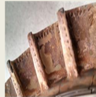
Typical build-up on blade
