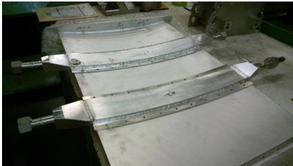
Figure 7: SLICE bolted channel test article.
