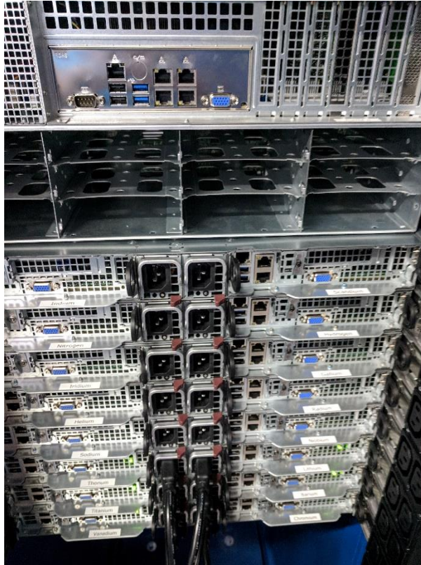
Figure 1. SOCRATES cloud-emulating computing hardware rack consisting of [currently] 16 computational nodes with 32 cores per node, used for the Spring 2018 Hindu Kush Himalayan Forecasting Experiment.
