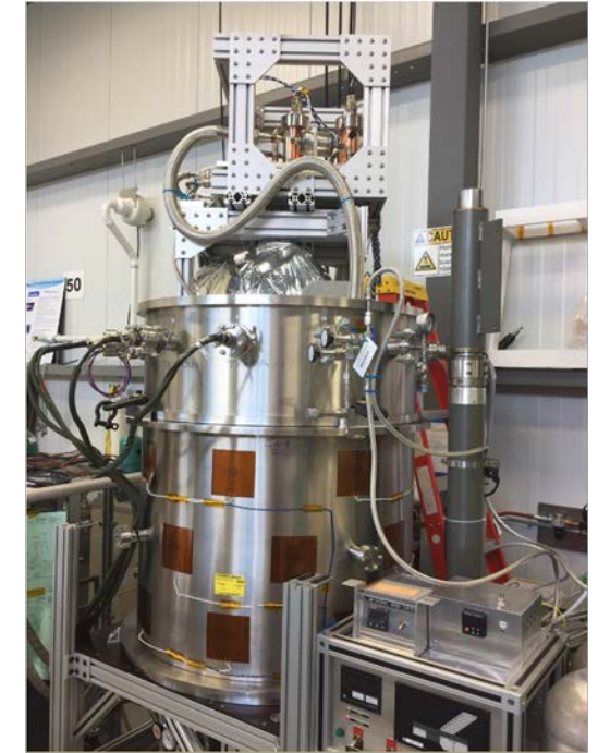
Figure 9. The assembled 20K-20W cryocooler installed into the bottom section of the vacuum bell jar, in preparation for testing.
