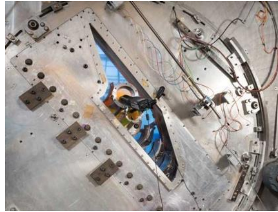
Figure 3. Endwall test section: a) heater strip locations; b) infrared window ports and cameras
