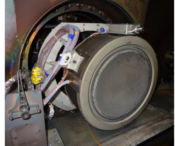
NEXT-C thruster development prototype
