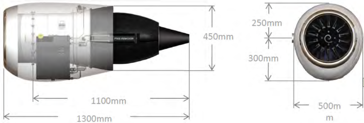
Figure 2. Price Induction DGEN380 Turbofan Engine Dimensions
