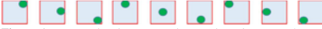
Figure 1 – Example of super-resolution algorithm using 9 input images, shifted from each other by a sub-pixel amount
